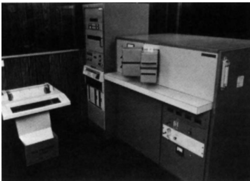
FIG. 24 —Optical Emission Spectrometer (OES) — Analysis of irons, production control samples and final product
