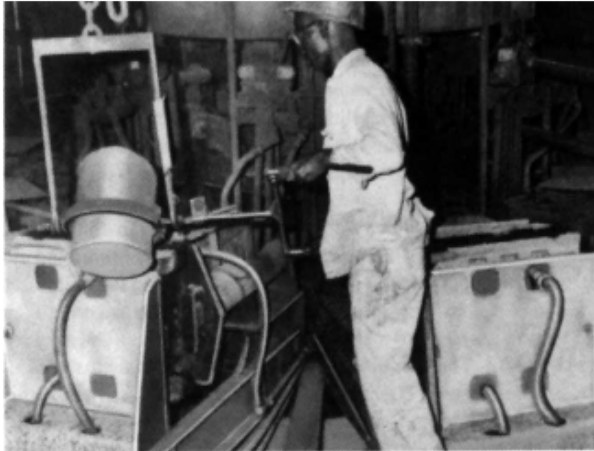
FIG. 14 — Rotating Wheel-Type Machine for Fittings Production
